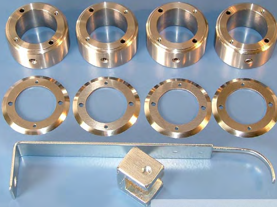
strip slitting ( gully cut ) unit complete
